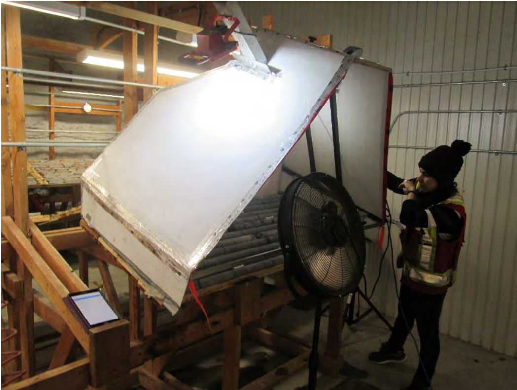
Figure 10-5: Core Photo Set-up; fan is used to dry core.
