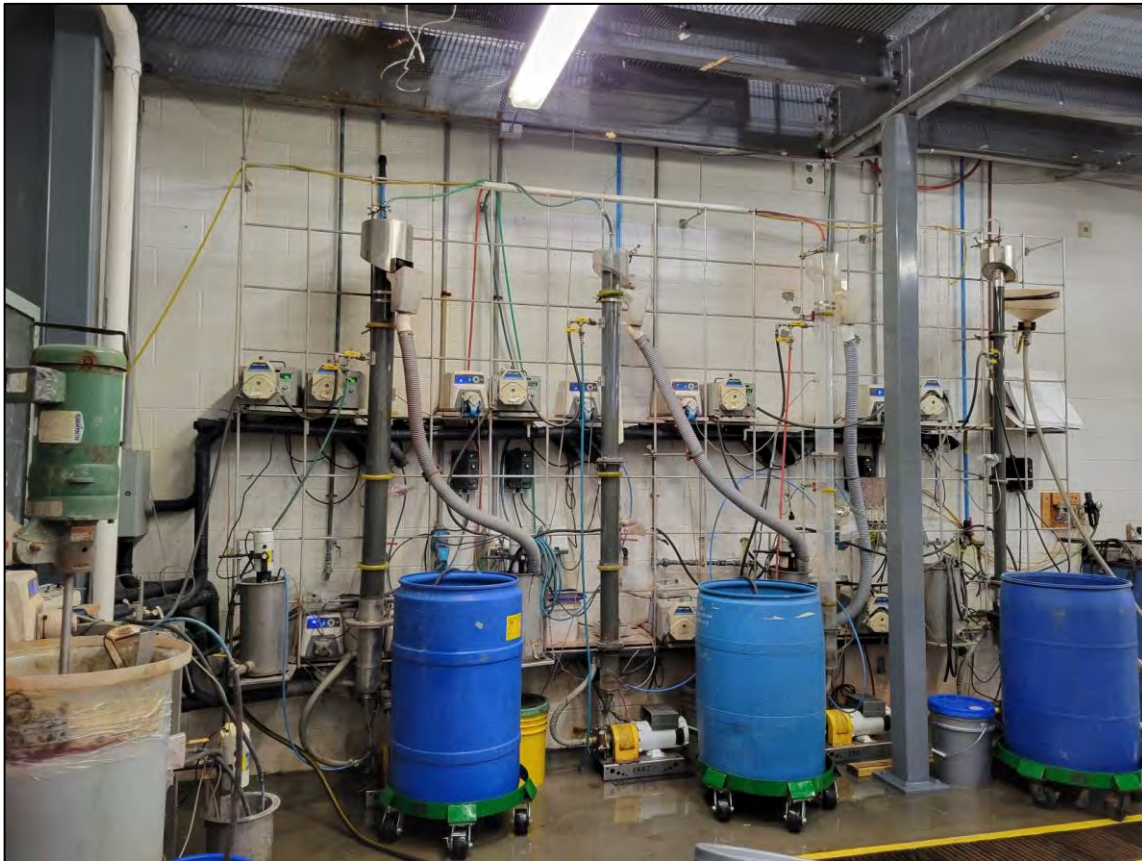
Figure 13-23: Eriez Pilot Plant 4” dia 1St Cleaner Column & 3”dia 2nd Cleaner Column & 2” 3rd Cleaner Column
