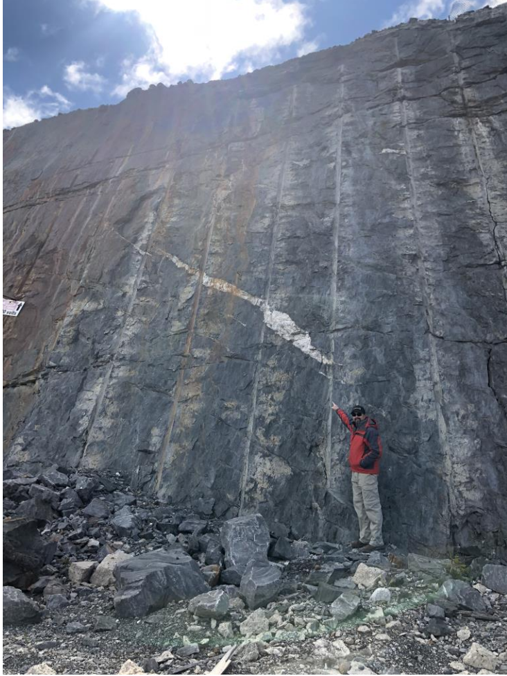
Figure 4: Example of the pinch and swell nature of quartz veining at Troilus in the Z87 pit wall
