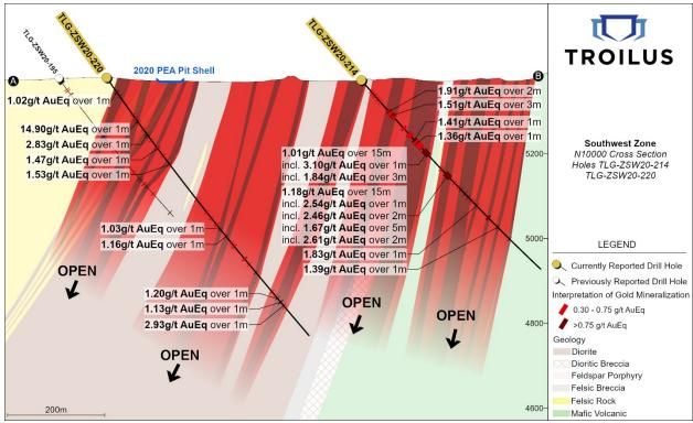
Figure 4: Section N10000; View of drill holes TLG-ZSW20-220 and TLG-ZSW20-214
