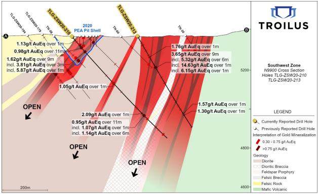
Figure 5: Section N9900; View of drill holes TLG-ZSW20-210 and TLG-ZSW20-213
