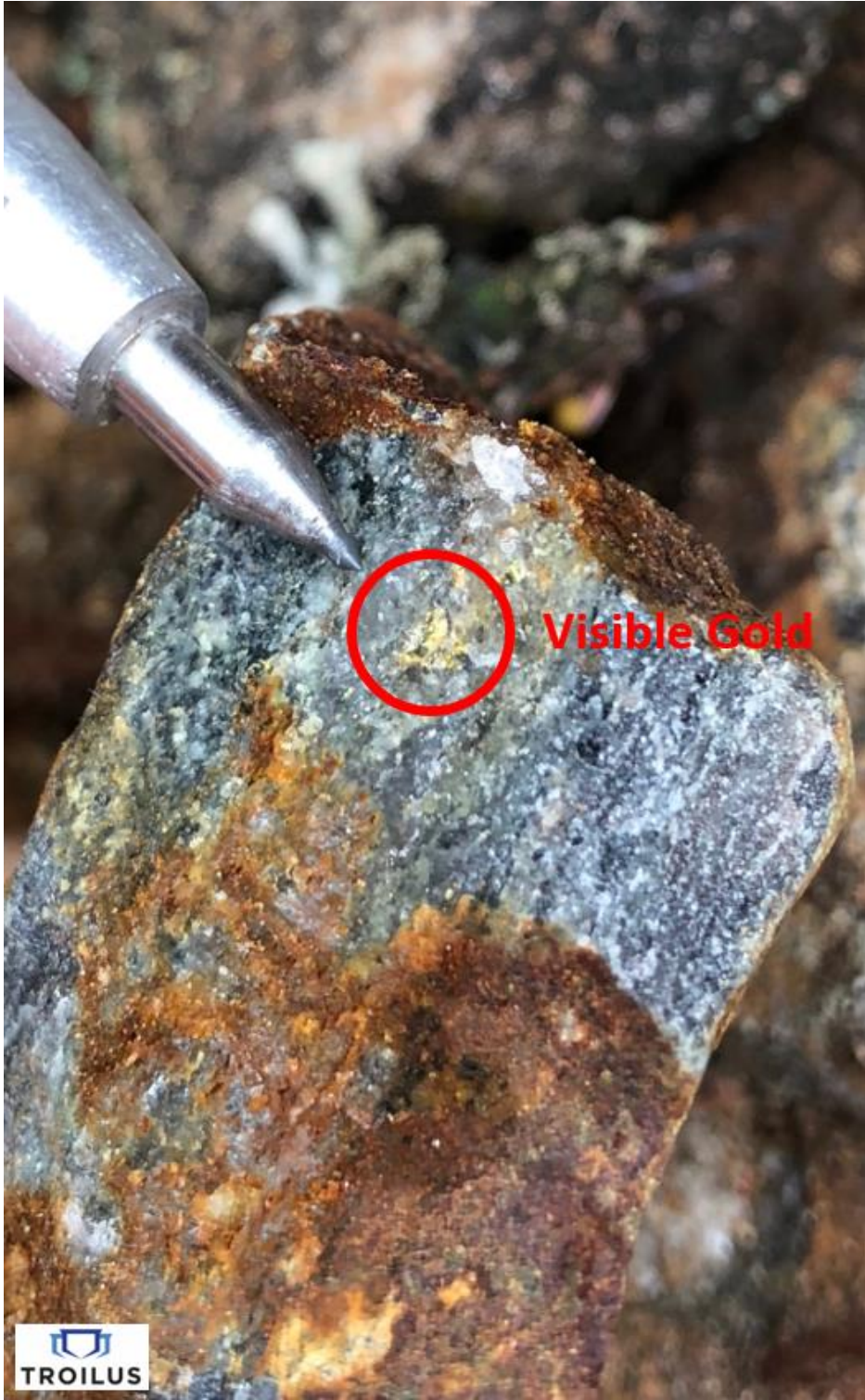
Image 1: Visible gold from sample TLG-TJ4N-18-JB-134 (110 g/t Au)
